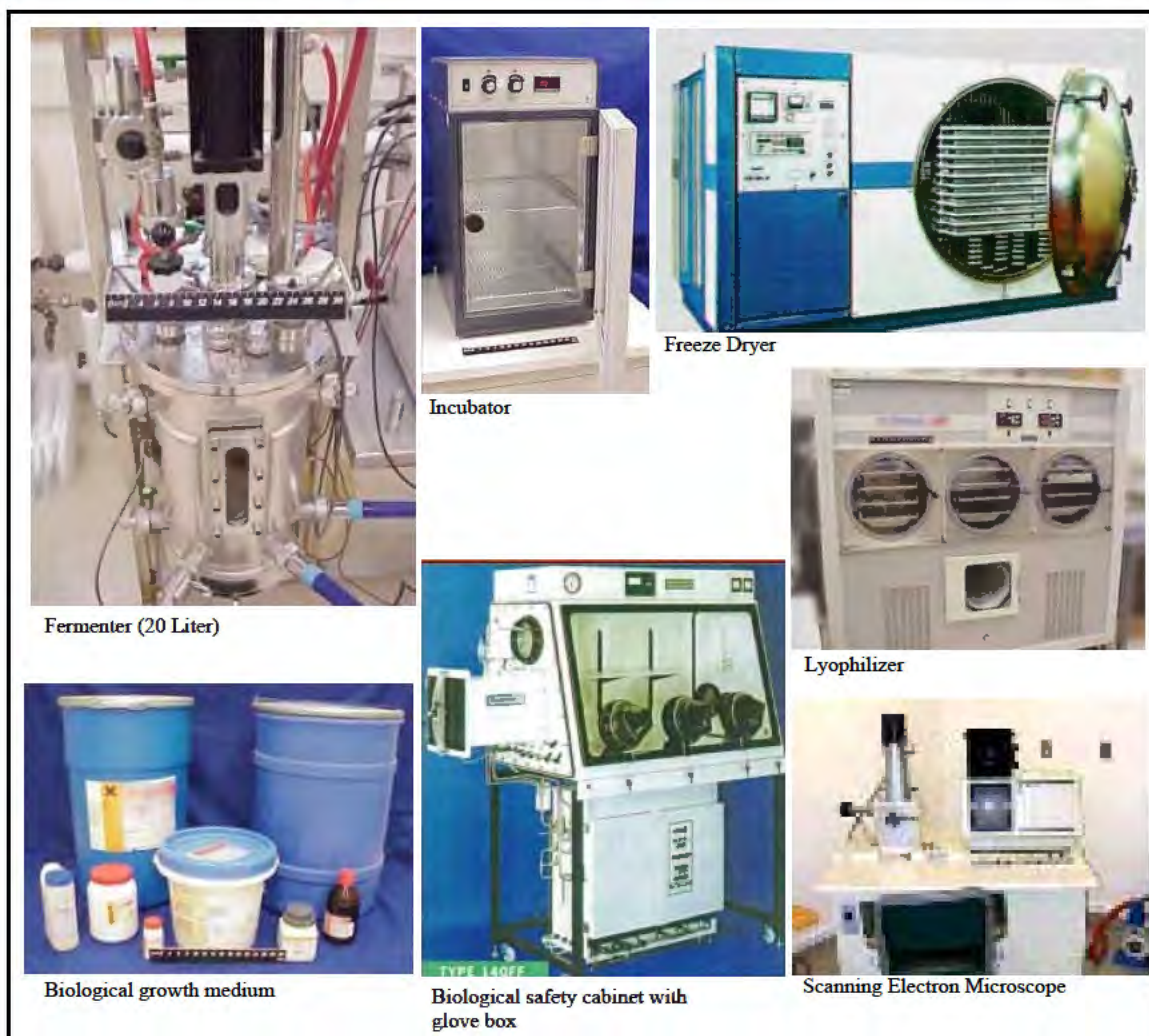
Figure 11. Types of Equipment Found in a Biological Weapons Laboratory.
