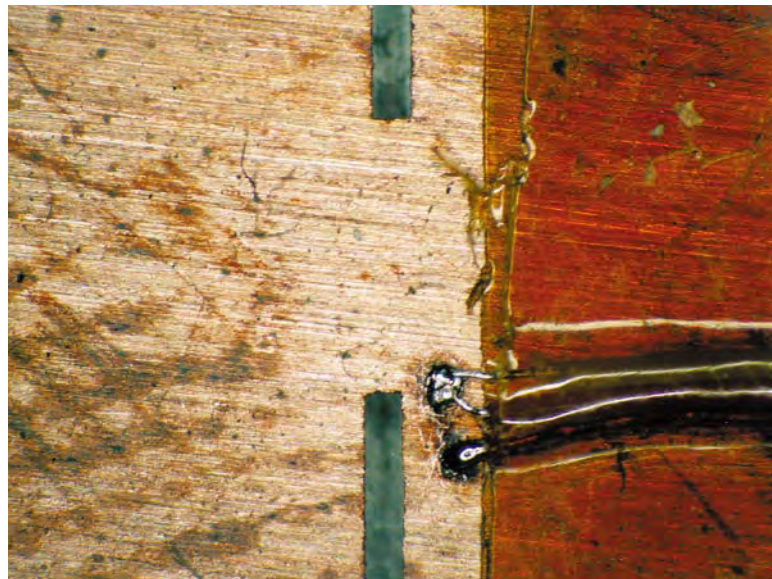
Figure 4. Photograph of test sample showing a 0.003-in.-diam thermocouple attached at the lower right corner of the sample gauge section.
