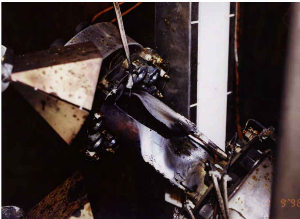
Figure 28. Aftermath of thermal explosion with LX-04 with 0.25 kbar confinement. The rupture was very mild, consistent with the radar data in Figure 27. One radar horn can be seen in the left of the photo, with the ruptured cylinder adjacent to it.
