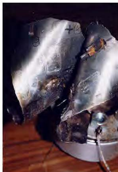
Figure 34. Ruptured vessel following PBX-9501 thermal explosion with 0.5-kbar confinement. Cylinder wall has been split and folded back on itself, but remains in one piece.
